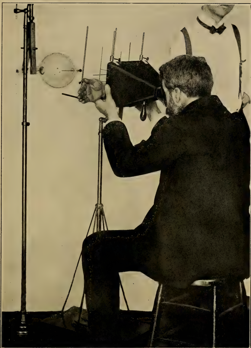
PLATE 65.—Author's One-Minute Localizer. Second Step. With all parts held as before simply give the entire frame, with screen and arm, a slight lateral turn to either right or left. Stop when the bullet has travelled over to the vertical guide. With the right hand slide the depthing rod straight back on its guiding rod till its marking pin is exactly over the shadow of the bullet on the vertical guide. The bullet is located by this simple method without any divergence or distortion whatever and in a single moment. Hold the part still in the frame, unclamp the fluoroscope, mark the point of the front marker on the skin and mark the skin where the pin of the depthing rod touches it. When the two cross sections are thus marked the surgeon will find the bullet at the intersecting point without deviation. Study these plates in connection with the descriptive text.
